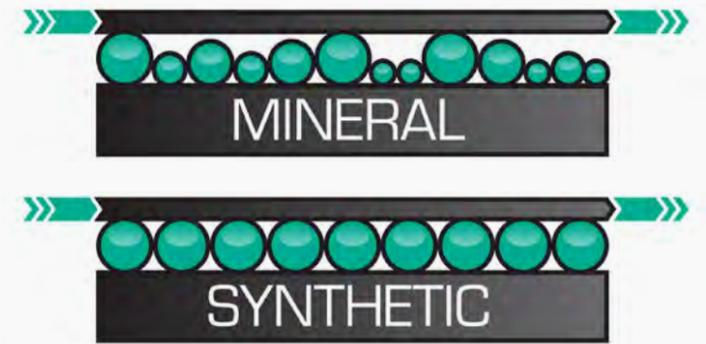
*Synthetic lubricants provide far more consistent lubrication compared to mineral oils due to increased uniformity in molecular structure.*
